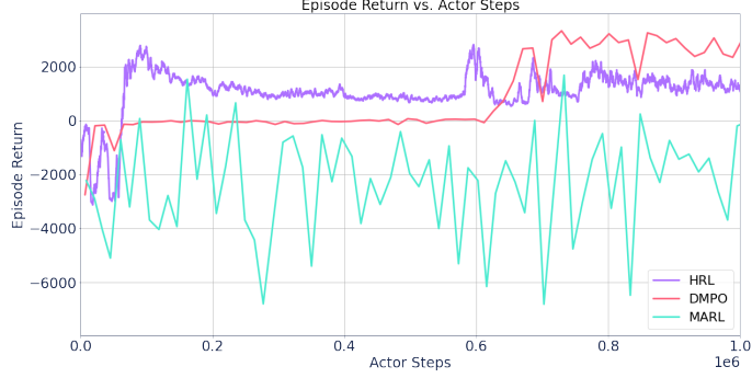
Figure 3: Episode return during first 1 million steps of training for DMPO, multi-agent RL and hierarchical RL agents. HRL is more sample efficient than DMPO, achieving higher reward within the first 100,000 steps. While DMPO converges to a higher episode return, this is due to DMPO manipulating chillers in an unsafe way to maximize the task balance reward. We constructed the reward function to see if any agent could learn safe and efficient chiller sequences and are more concerned with downstream behavior than episode return.
