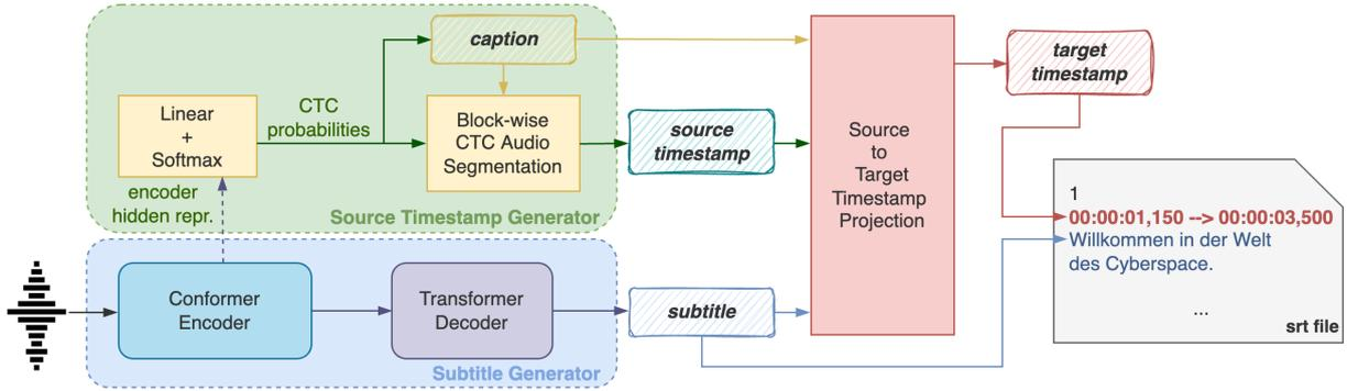
Figure 1: Architecture of the direct ST system for automatic subtitling.
