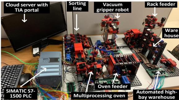
Figure 6: A small scale real-world testbed of automated high-bay warehouse to evaluate *BayesImposter*.
