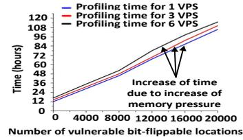
Figure 9: Profiling time for different number of VPSs.
