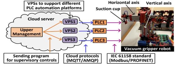
Figure 1: Different components of an ICS in cloud settings.
