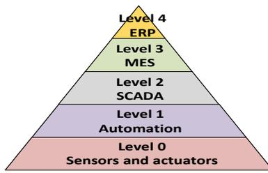
**Figure 11: Automation pyramid in a typical Industry.**
