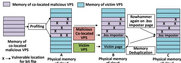
**Figure 5: (A) Profiling the memory of cloud. (B) Placing .bss imposter page in the vulnerable location. (C) After memory deduplication, victim page is backed by the .bss imposter page and the Rowhammer causes bit flips in the .bss imposter page.**
