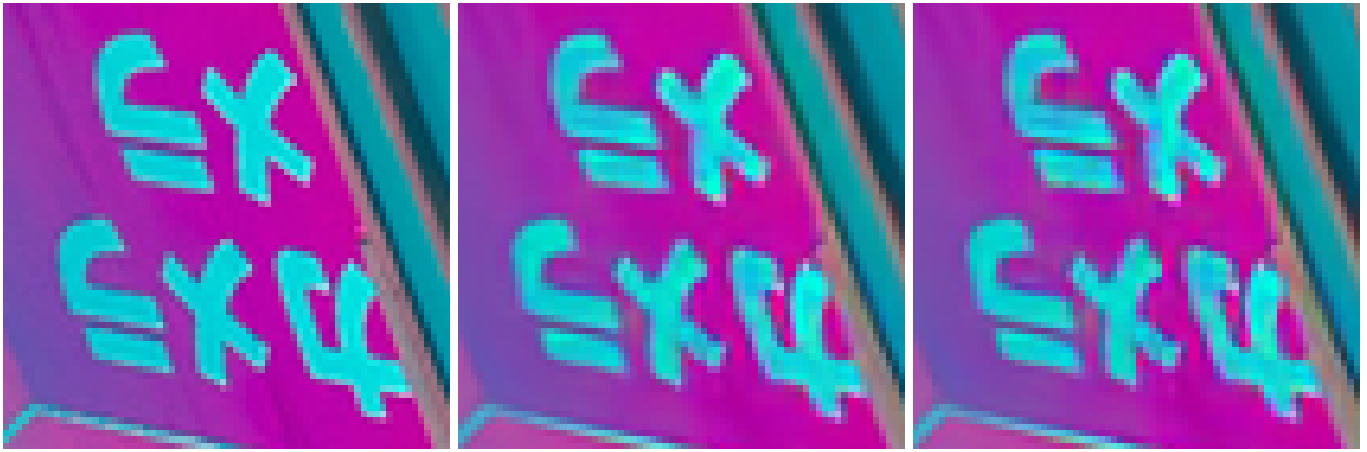
Fig. 4. Illustration of our approach on image 22 of the CLIC Test Set for cheng2020-anchor : the original (left), ours (middle) and the corresponding unimproved baseline (right). The figure shows only a patch of the image.
