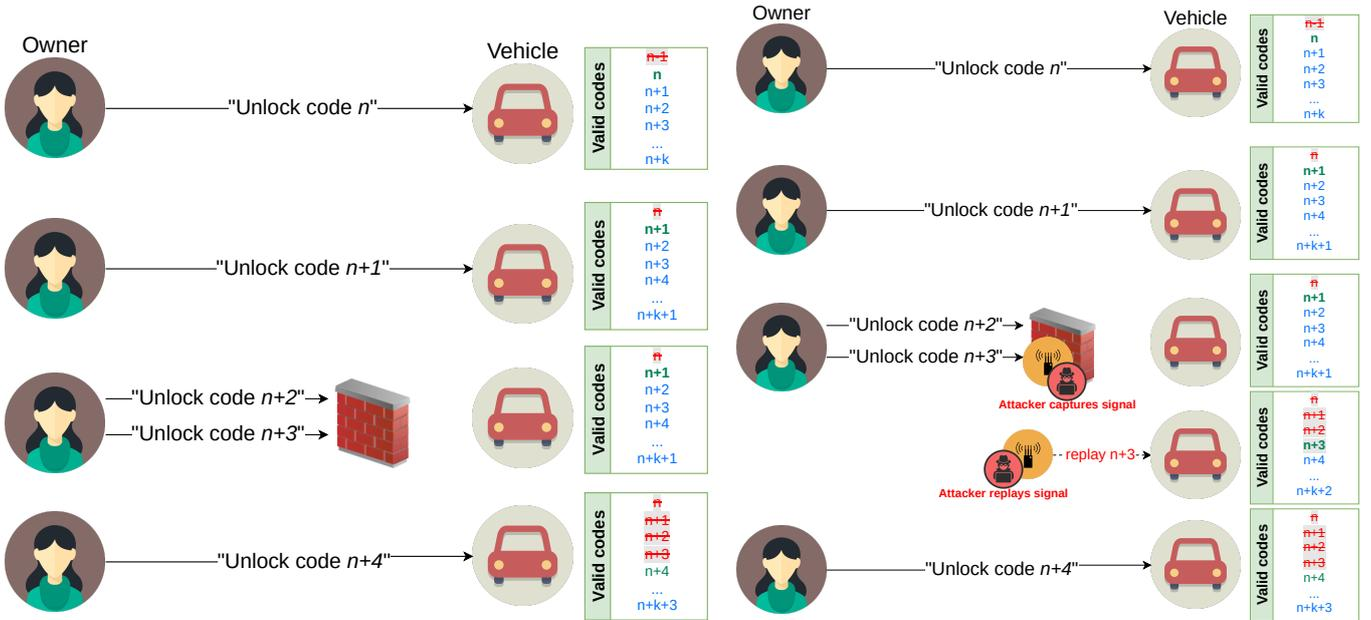
(a) Essence of rolling codes: every signal is unique and (b) “Straightforward exploit” of the safety feature in rolling code-based systems gets invalidated by the next one.
