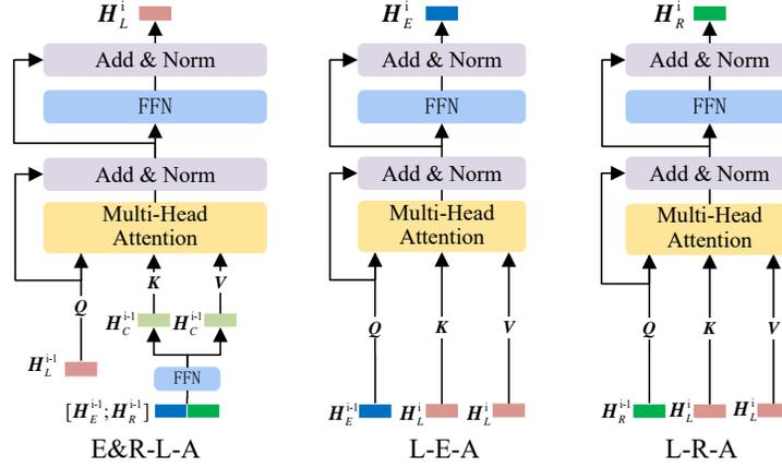
**Figure 3** Neural architectures of E&R-L-A, L-E-A, and L-R-A. The three units share a common architecture but differ in inputs.
