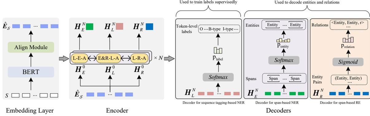
**Figure 2** The illustration of STSN, which consists of a BERT-based embedding layer, an encoder and three separate linear decoders. We solely use the decoder for sequence tagging-based NER to train token-level label semantics ( $H_L$ ) in a supervised way. And entities and relations decoded by the span-based NER and RE decoders are used to evaluate model performance.
