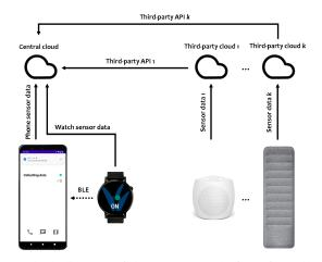
Fig. 1: Block diagram of the MAISON platform for collecting data from phones, watches, and external sensors, see Section III.
