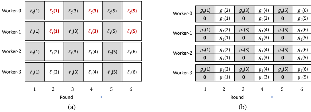
Figure 12: Consider parameters \{n = 4, B = 1, W = 2, \lambda = 4\} ; (a) SR-SGC scheme: reattempted tasks are indicated in red (b) M-SGC scheme.
