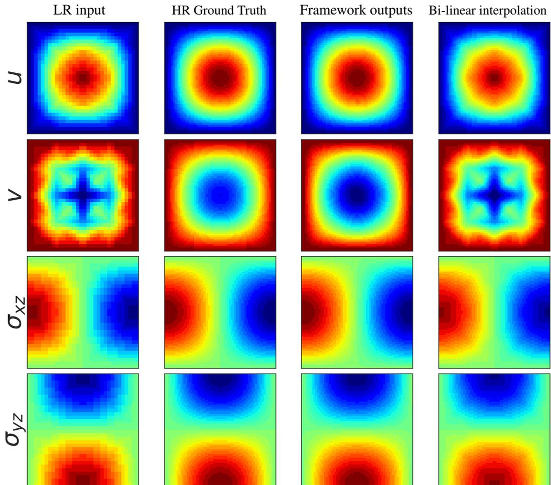
Figure 6: The figure shows the snapshot of the elastodynamics' solution fields at a time step. The LR input and HR Ground-truth are the coarse-scale and fine-scale solution fields obtained using the finite element method. For a given LR input, the reconstructed solution from the framework is highly accurate compared to the bi-linear interpolation method.
