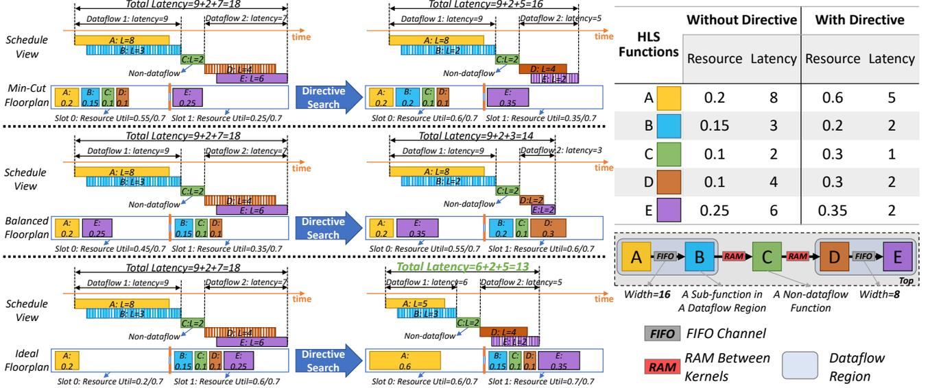
**Figure 2: A Toy Example with 2 Dataflow Kernels and 1 Non-dataflow Kernel, with Different Latency (L) and Resource Consumption (R). Three Different Floorplanning Methods and the Corresponding DSE Results Are Compared.**
