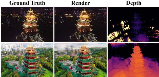
Figure 6. Different scans of the same scene during day and night. Both RGB and depth images are synthesized by Mega-NeRF [35].
