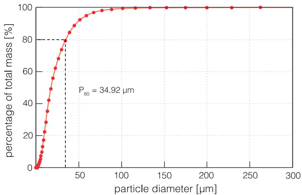
**Figure S2. Cumulative particle size distribution of basalt feedstock.** Determined by laser diffraction particle size distribution analysis.
