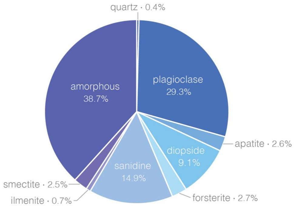
**Figure S3. Mineralogy of basalt feedstock.** Determined by X-Ray diffraction analysis.
