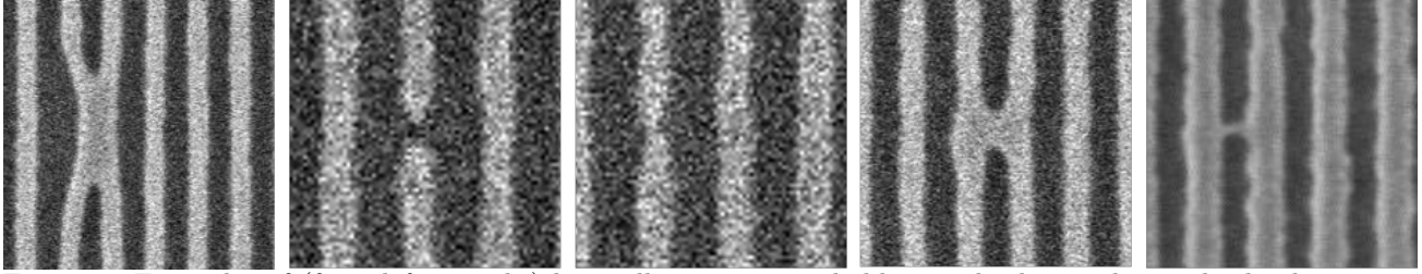
Figure 1: Examples of (from left to right) line collapse, gap, probable gap, bridge, and microbridge line space pattern defects.
