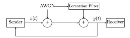
Figure 1: The continuous-time ARMA(1,1) Gaussian channel with feedback. Note that the OU process  $\{u(t)\}$  can be interpreted as the white Gaussian noise  $\{w(t)\}$  filtered by a Lorentzian filter (see, e.g., [35]).
