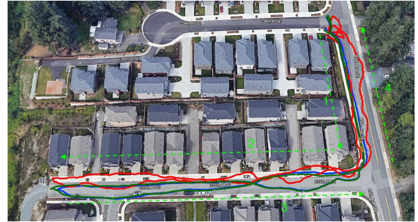
Fig. 1: Demonstration of GNSS pseudorange trajectory (red), GNSS carrier-phase trajectory (green) and VIO trajectory aligned with GNSS carrier-phase in the first 50 m (blue). The light-green numbers and dashed lines indicate the direction of four major parts of the trajectory. We can observe that the pseudorange trajectory is much noisier than the other two with a positioning error of up to 10 m. This indicates the potential of GNSS carrier-phase for more precise global positioning than GNSS pseudorange.
