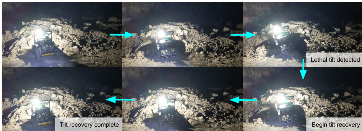
Figure 12: Tilt recovery behavior when the robot pitch exceeds the safe limit.
