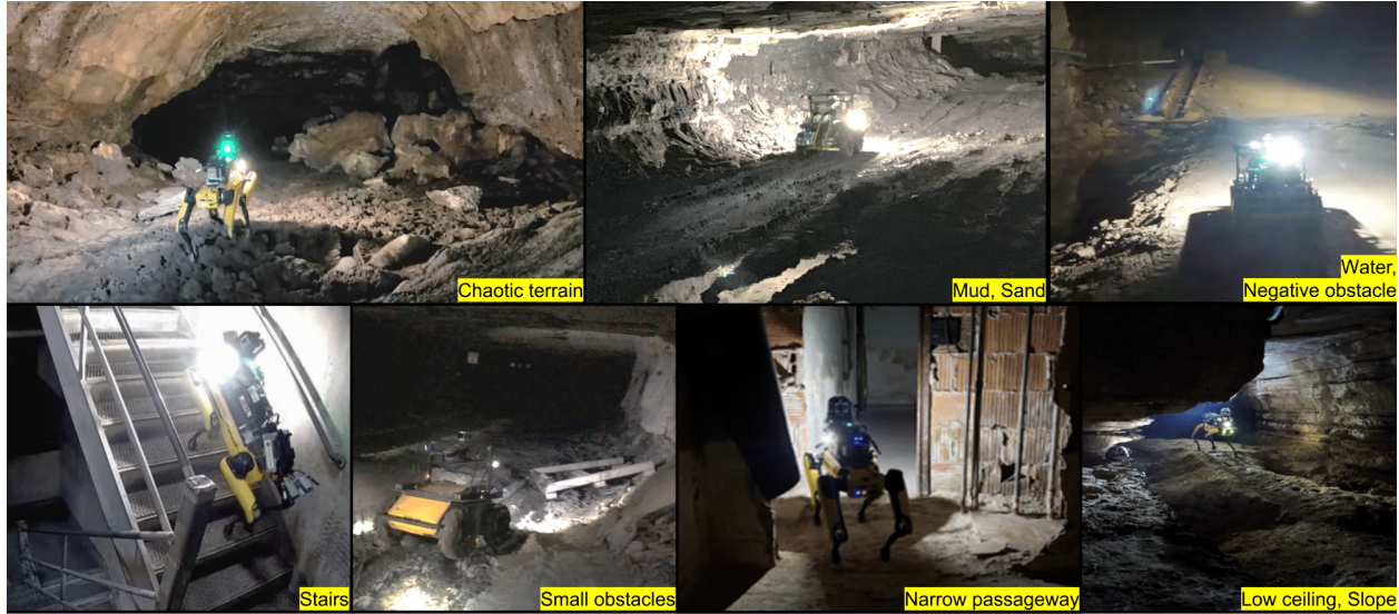
Figure 1: Top left: Boston Dynamics Spot quadruped robot exploring Valentine Cave at Lava Beds National Monument, CA. Top middle, bottom middle (second image from the left): Clearpath Husky robot exploring Arch Mine in Beckley, WV. Bottom left: Spot exploring abandoned Satsop power plant in Elma, WA.
