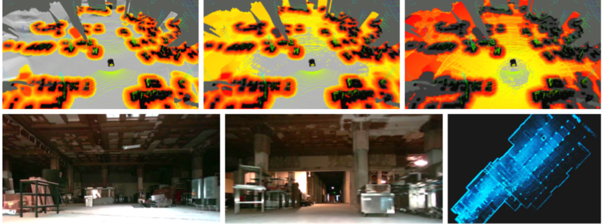
Figure 15: Traversability analysis results for Husky in an abandoned subway experiment. Top left to right: Risk maps at three varying risk levels: \alpha=0.1 , 0.5 , 0.9 , respectively. Colors correspond to CVaR value (white: safe ( r \leq 0.05 ), yellow to red: moderate ( 0.05 < r \leq 0.5 ), black: risky ( r > 0.5 )). Also shown are the most recent LiDAR measurements (green points). Bottom left and middle: Front and right on-board cameras observing the same location. Bottom right: Completed top-down map of the environment after autonomous exploration. Bright dots are pillars, which are visible in the camera images. The effect of these risk analyses results in intuitive outcomes - for example, a low pile of metal, while probably traversable, should be avoided if possible. When the region has inadequate sensor coverage, the risk will be high. When the robot is closer and the sensor coverage is good, then the CVaR cost will decrease, yielding a more accurate risk assessment. This results in more efficient and safer planning when compared to deterministic methods.
