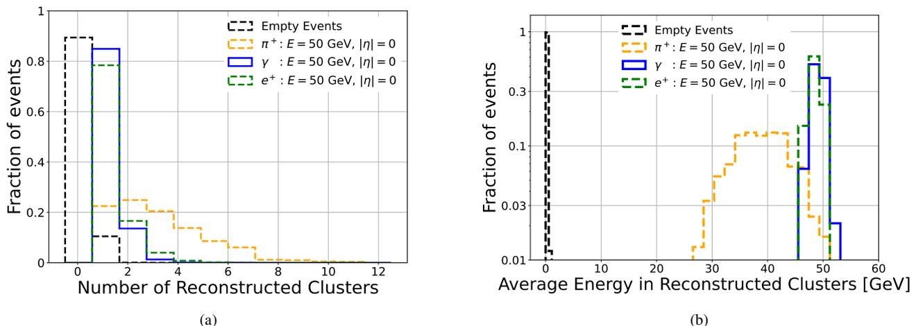
Fig. 5: Number (a) and average energy (b) of reconstructed clusters in COCOA for events with a single charged pion, electron, or photon shot at  $\eta = 0$ . Results are also shown for clusters reconstructed in empty events due to electronic noise. The default topological calorimeter cell clustering settings are used.
