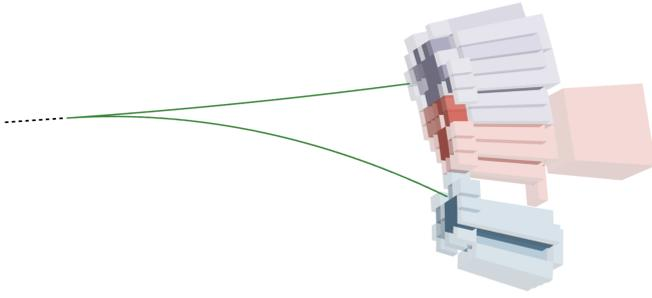
Fig. 1: Visualization of a photon (dashed line) with energy 50 GeV converting to two electrons (green lines) producing three distinct clusters in the COCOA central electromagnetic calorimeter. The cluster shown in red contains an additional cell in the first layer of the hadronic calorimeter due to a noise fluctuation. Cells are shown with an opacity proportional to energy over noise ratio divided by 4.6, the threshold for topoclustering seeds.
