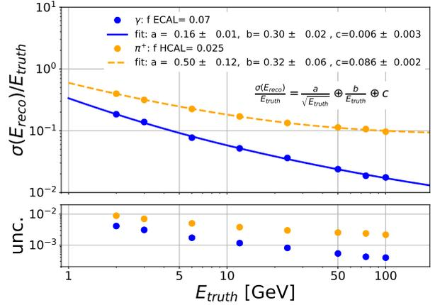
Fig. 9: The relative energy resolution  $\sigma(E_{\text{reco}})/E_{\text{truth}}$  is plotted as a function of  $E_{\text{truth}}$  for eight different truth energy values and fitted with the relative-resolution function, for photon and pion, respectively. The average sampling fraction  $f$  for ECAL and HCAL are shown in the legend.
