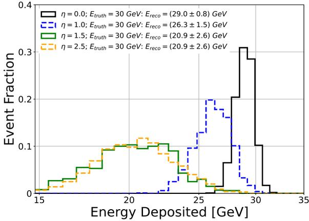
Fig. 8: Reconstructed energies of electrons with an energy of 30 GeV for different directions  $\eta$ . As the initial electron momentum is directed closer to the beamline, the difference between the reconstructed energy and the initial particle energy increases due to the iron traversed by the electron upstream the calorimeter (dead material).
