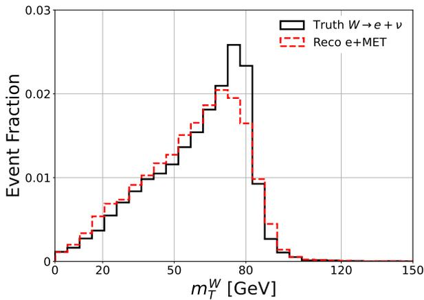
Fig. 10: The transverse W mass  $m_T^W$  distribution is plotted for leptonically decaying W events. The black curve shows the truth distribution whereas the red curve is obtained from the vector sum of reconstructed lepton momentum and the MET in the event. The peak location of the two distributions are well aligned, demonstrating that the event-level reconstructed MET is trustworthy within the COCOA framework.
