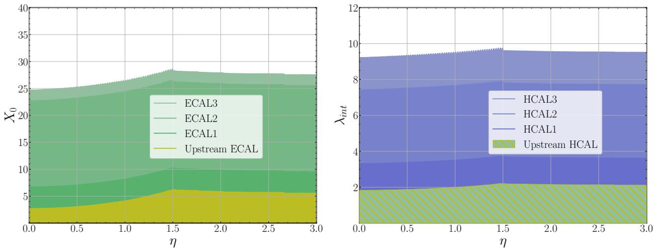
Fig. 3: (left) Cumulative amounts of material, in units of radiation length  $X_0$  and as a function of  $\eta$ , in front of and within the electromagnetic calorimeter system. (right) Cumulative amounts of material, in units of interaction length  $\lambda_{int}$  and as a function of  $\eta$ , in front of and within the hadronic calorimeter system.
