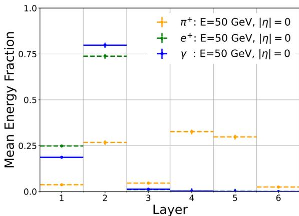
Fig. 6: Energy deposited by electrons, photons and charged pions for each calorimeter layer. The electron and photon showers are limited to the electromagnetic calorimeter (layers 1 to 3) while the charged pion showers reach deep into the hadronic calorimeter (layers 4 to 6)
