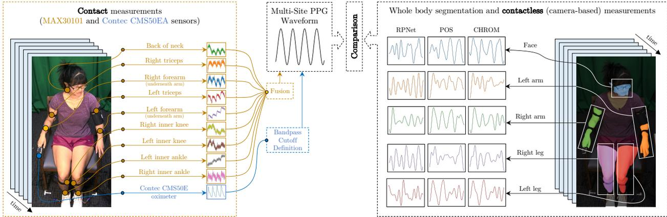
Figure 1. This paper explored the (a) Multi-Site Physiological Monitoring (MSPM) dataset with **contact** measurements from ten PPG sensors, including a fingertip oximeter, as shown on the left, with (b) **contactless** (camera-based) measurements of multiple skin areas carried out by three state-of-the-art rPPG methods (CHROM [9], POS [44], and RPNet [36]) as shown on the right. In this paper we also compared de-noised and combined PPG signals with the corresponding rPPG estimates.
