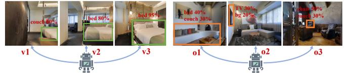
Fig. 1. The illustration of semantic distribution disagreement, e.g., the bed is recognized to different objects/distributions across three viewpoints ( $v_1, v_2, v_3$ ), and semantic distribution uncertainty, e.g., the probability of couch in observation  $o_1$  being predicted as bed and couch is relatively close. bg means background.
