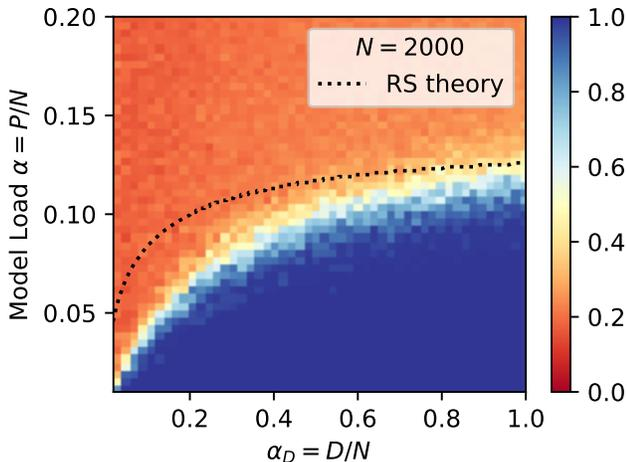
FIG. 2: Comparison with numerical results for the retrieval of one pattern. Each pixel represents the mean pattern magnetization for given values of  $\alpha$  and  $\alpha_D$ , averaged over 25 samples of size  $N = 2000$ . The simulations are performed initializing the model to a pattern  $\xi_\nu$ , running the update rule (4), then measuring  $m_\nu$  at convergence.
