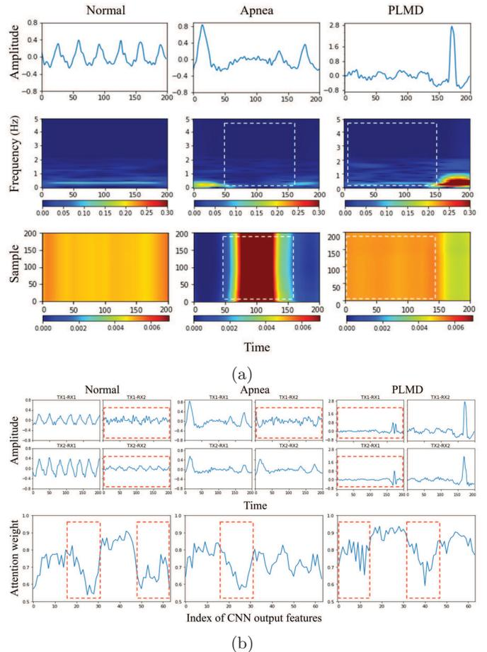
Fig. 4: The observation of attention weights of (a) time attention in GRU and (b) antenna-pair attention (Note that indexes of attention weights from 1-16 stands for pair 1, 17-32 for pair 2, 33-48 for pair 3 and 49-64 for pair 4).
