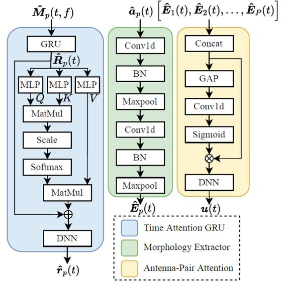
Fig. 3: Neural network model for ALESAL. "MatMul" denotes inner product of two matrices. "BN" stands for batch normalization. "GAP" and "Conv1d" respectively indicate the operation of global average pooling and 1D convolution.
