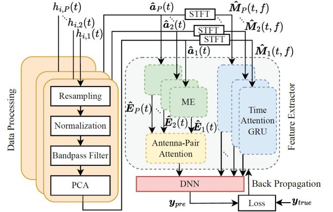
Fig. 2: Schematic diagram of the proposed ALESAL system.
