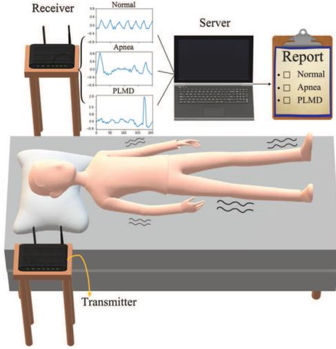
Fig. 1: System architecture for contactless sleep apnea and PLMD detection using commercial Wi-Fi CSI signals.
