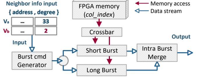
**Figure 8: Hardware architecture of dynamic burst engine.**
