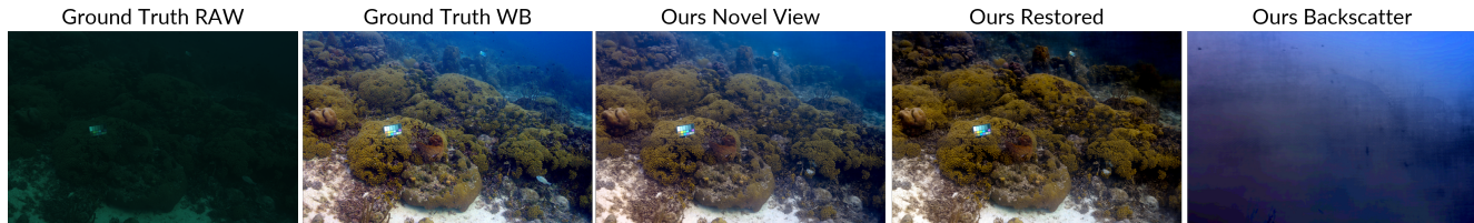
Figure 1. NeRFs have not yet tackled scenes in which the medium strongly influences the appearances of objects, as in the case of underwater imagery. By incorporating a scattering image formation model into the NeRF rendering equations, we are able to separate the scene into ‘clean’ and backscatter components. Consequently, we can render photorealistic novel-views with or without the participating medium, in the latter case recovering colors as if the image was taken in clear air. Results on the Curaçao scene: A RAW image (left) is brightened and white balanced (WB) for visualization, showing more detail, while areas further from the camera (top-right corner) are occluded and attenuated by severe backscatter - which is effectively removed in our restored image. Please zoom-in to observe the details.
