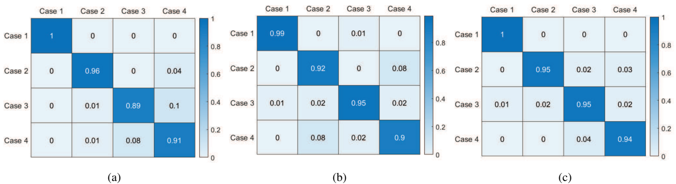
Fig. 10: Confusion matrix of ALPD in the normal state using (a) pair 1, (b) pair 2 and (c) both pairs with average accuracy of 94%, 94%, and 96%, respectively.
