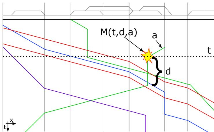
**Figure 7:** Malfunction generation. This figure illustrates a simple operations plan with 6 trains on a small infrastructure. A single malfunction  $M(t, d, a)$  occurs for train  $a$  at time  $t$  with a total duration of  $d$  time steps.
