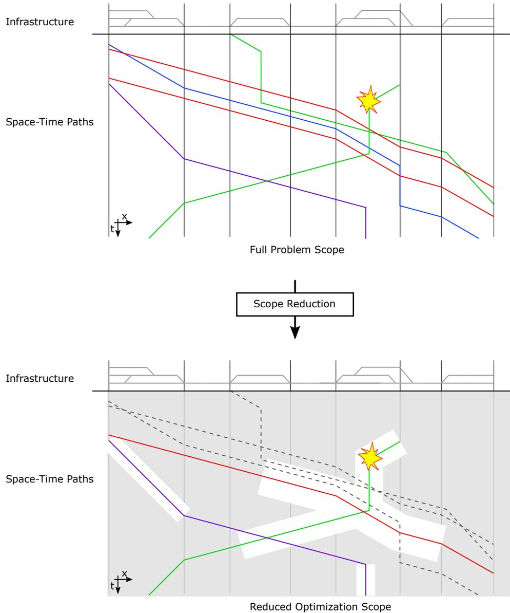
**Figure 3:** Illustration of scope restriction. The aim is to vastly restrict the search space of an optimizing algorithm, condensing the initial full problem description to the core problem in the time-space parameters.
