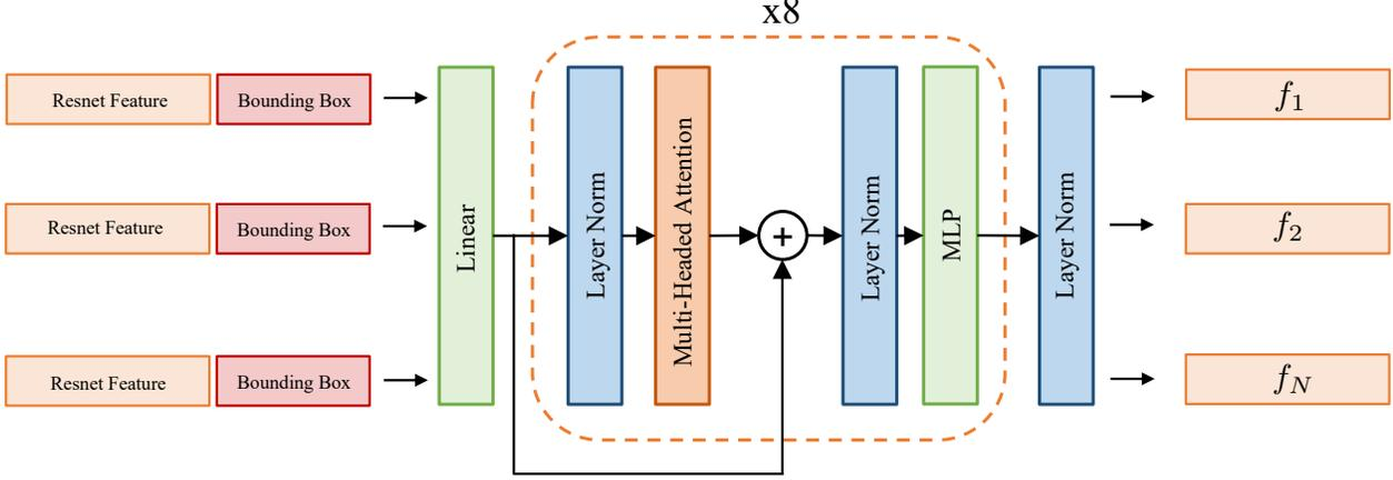
Figure 10. **Encoder Architecture Diagram** Our transformer encoder takes as input a set of  $N$  Resnet image features concatenated with the bounding box information for that image. After 8 layers of 12-headed self-attention and a final Layer Normalization layer, we receive output features  $f_1 \dots f_N$ . Unlike the input Resnet features, each of these features  $f_1 \dots f_N$  depends on every image in the set.
