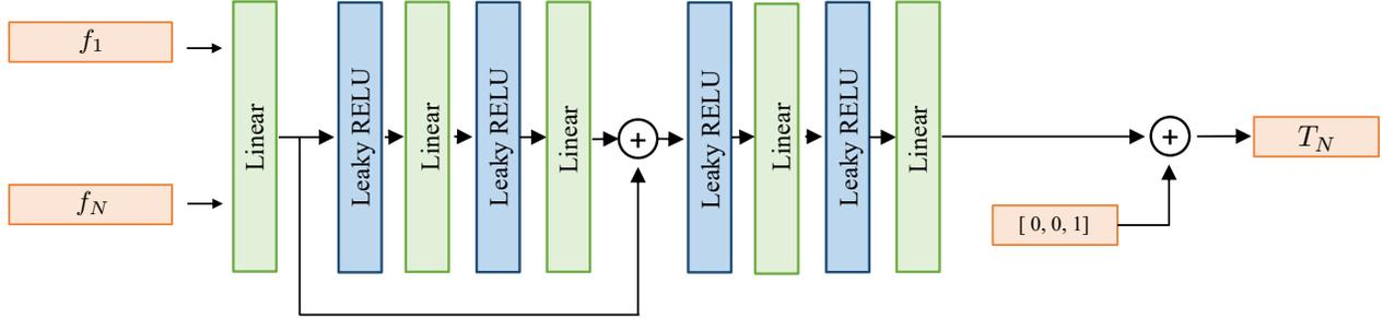
Figure 11. **Translation Regressor Architecture Diagram** For regressing to  $T_N$ , we concatenate transformer features  $f_1$  and  $f_N$  as input to the translation regressor network. We choose to include  $f_1$  as input since the scale of the scene is determined by the first image (the norm of the translation target for the first camera is always set to 1).
