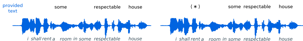
Figure 5: Illustration of the \langle * \rangle Token in Forced Alignment. We show the text to which we would like to align the audio at the top and what is actually spoken at the bottom in italics. Left: erroneous alignment when the provided text is incomplete. The word some is aligned incorrectly. Right: using \langle * \rangle token at the beginning enables correct alignment of the provided text.
