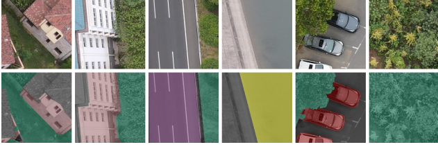
Figure 8. Class definition in the VDD dataset. From left to right: roof, wall, road, water, vehicle, and vegetation. Note that we label images in pixel-level. This figure is a close look of annotations in VDD.
