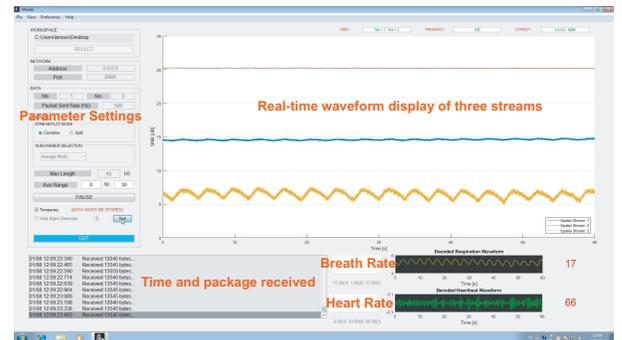
Fig. 9: Real-time system interface. The upper left part is the parameter setting interface, which can be used to set the storage location of the received data, the time axis scale, the receiving rate, the sender’s IP address, whether to enable vital sign detection, etc. The bottom left shows the time when the current packet was received and the size of the packet. The top right is the real-time display of the CSI waveform, and the bottom right is the real-time display of vital signs.
