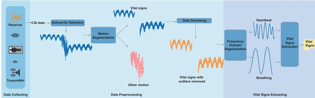
Fig. 5: System architecture.
