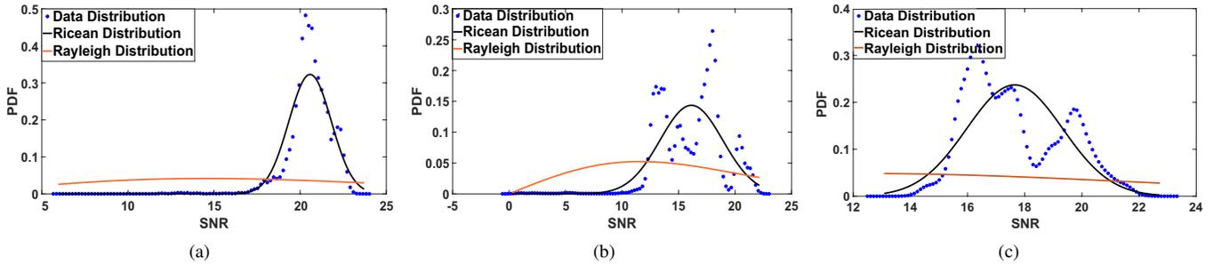
Fig. 17: Distributions of the three streams in Fig. 3a. (a) T1–R1,  $K = 201.1$ . (b) T1–R2,  $K = 17.8$ . (c) T1–R3,  $K = 52$ . PDF means probability density function.
