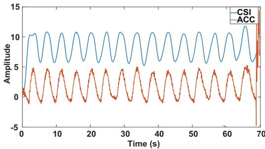
Fig. 14: Comparison of the processed CSI and the accelerometer (ACC) readings for breathing.
