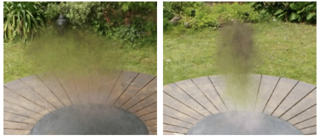
Figure 4. Examples of artifacts in the initialized NeRF. 2D inpaintings contain inconsistent inpainted pixels that accumulate in the 3D inpainted region and appear as floater artifacts.
