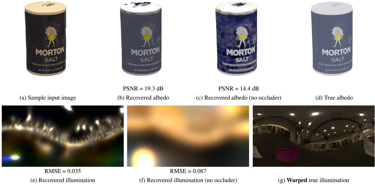
Figure 8. Results on the captured `salt004` scene from Stanford-ORB [18]. Note that the “warped true illumination” environment map (g) was captured by a light probe that was not co-located with the object, any may therefore be significantly warped. The recovered RMSE reported is computed with respect to the average of all environment maps provided with the dataset rotated the same coordinate frame.
