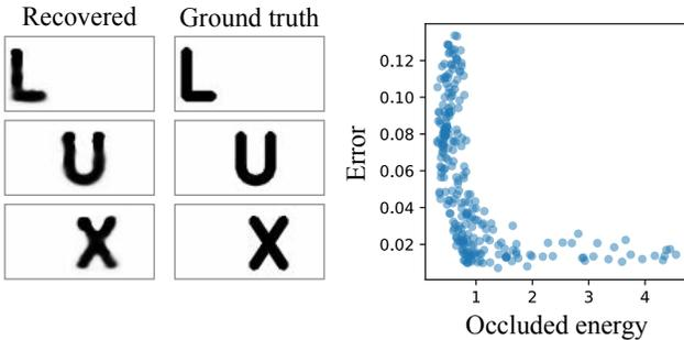
Figure 5. Our occluders extracted from the *potatoes* scene on the top of Figure 4 resemble the true ones (left). However, as expected, inaccuracies in the recovered masks tend to occur at relatively-dark regions of the environment map: there is a very strong inverse correlation (right) between the mean error in the recovered masks and the amount of illumination energy that they block.
