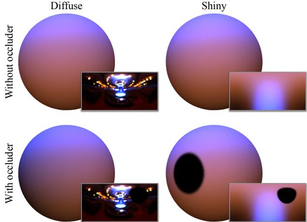
Figure 2. Decomposing appearance into lighting and materials can be inherently ambiguous. Top row: a diffuse sphere lit by high-frequency lighting (inset) is visually indistinguishable from a shiny, mirror-like sphere lit by low-frequency lighting. Bottom row: A second image captured in the presence of a dark external occluder resolves the ambiguity. The occluder’s effect is clearly visible on the shiny sphere while on the diffuse sphere it produces shadows that are soft and very subtle.
