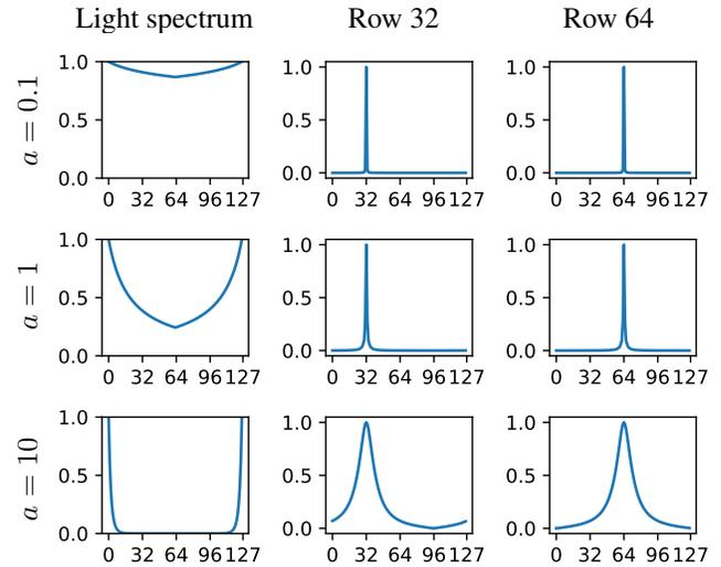
Figure S8. Most of the energy of the matrix  $B$  is concentrated around the diagonal elements in the Fourier basis. Each row shows, from left to right: the incident illumination spectrum (which modifies  $B$ ), and the magnitude of the elements of the 32nd and 64th rows of  $F B T^\top$ , where  $F$  is the DFT matrix. Each row corresponds to a  $1/f^a$  spectrum for  $a = 0.1, 1, 10$ . See text for more details.
