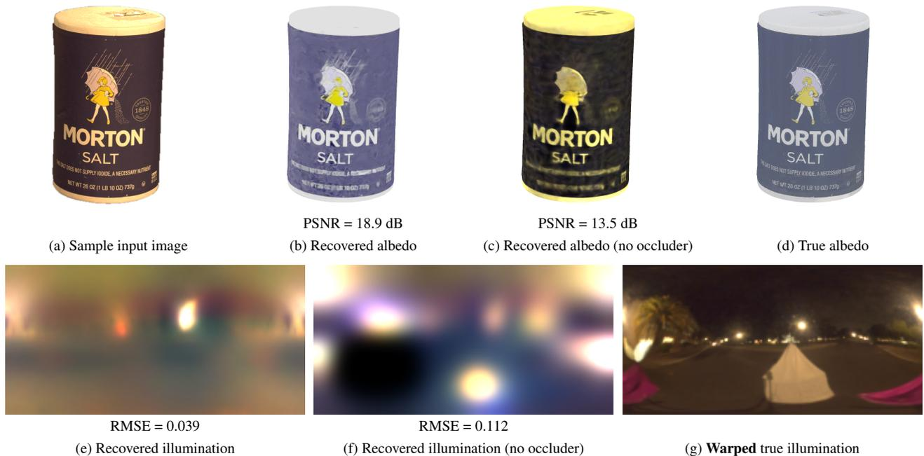
Figure S2. Results on the captured `salt007` scene from Stanford-ORB [18], extending Figure 8 of the main paper. Note that the “warped true illumination” environment map (g) was captured by a light probe that was not co-located with the object, any may therefore be significantly warped. The recovered RMSE reported is computed with respect to the average of all environment maps provided with the dataset rotated the same coordinate frame, see text and Figure S7.
