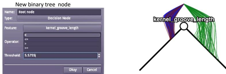
(a) Setting up the root threshold and operator,
