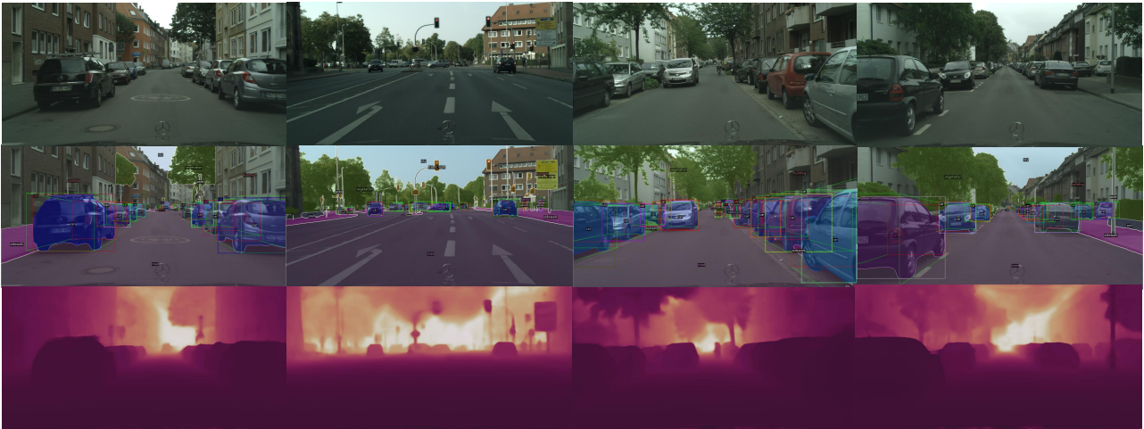
Fig. 6 Qualitative analysis of our multi-task results on Cityscapes validation set. The first row is raw images and the last two rows are our multi-task predictions. Best viewed in color and zoom in.
