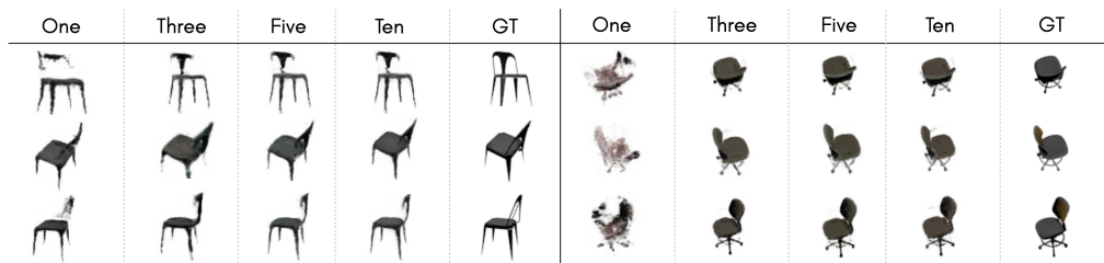
Figure 10: Multiview test-time optimization on SRN Chairs. HyP-NeRF can perform test-time optimization (see main paper, Section 3.1) with any number of views. In this qualitative result, we start with an instance that did not optimize well through a single pose (because of a challenging viewpoint) and show the improvement in quality of the generated NeRF as we increase the number of views (ie. coverage) for optimization. The header indicate the number of views used for the optimization. As shown, the difference in quality between five and ten poses is insignificant. The rightmost result shows drastic improvement in the render quality from one to three views showcasing the impact of pose on test-time optimization.
