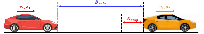
Fig. 5. Two vehicles driving in the same direction: red vehicle (rear) drives at (v_1, a_1) ; orange vehicle (front) drives at (v_2, a_2) .
