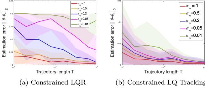
Fig. 1. The figures plot the estimation error of  $\tilde{\theta}$  when applying  $u_t = \pi_{\text{RMPC}}(x_t) + \eta_t$  under different excitation levels  $\sigma_\eta$ . Figure (a) considers the constrained LQR in (6), so  $\pi_{\text{RMPC}}(x_t)$  is time-invariant. Figure (b) considers a time-varying tracking problem, so  $\pi_{\text{RMPC}}(x_t)$  is time-varying. The solid lines represent the sample mean. The shades represent one standard deviation.
