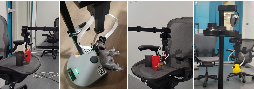
Figure 15: Grasping tests in various lab environments. To provide a strong baseline, we tuned the grasp policy to be highly reliable given the Stretch’s viewpoint, on a variety of objects.
