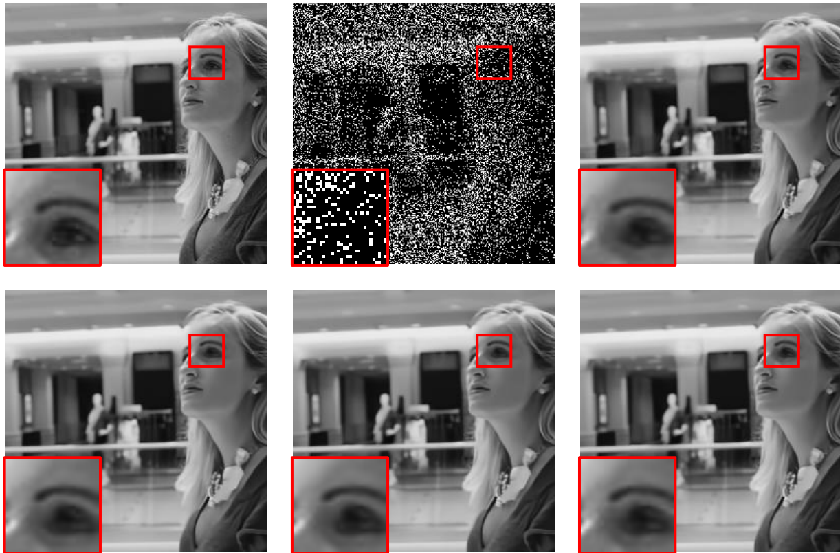
Fig. 6. Subjective quality of scene reconstruction and compression. Top left: GT scene frame. Top middle: GT spike frame. Top right Reconstruction scene frame via VTM (BPP=0.35,PSNR=36.42dB). Bottom left: Reconstruction scene frame via Baseline (BPP=0.33,PSNR=37.29dB). Bottom middle: Reconstruction scene frame via Baseline with SOAM (BPP=0.33,PSNR=37.35dB). Bottom right: Reconstruction scene frame via Baseline with BiSOAM (BPP=0.34,PSNR=37.44dB). Results show our proposed method outperforms conventional and learning-based codecs, reaching SOTA performance.
