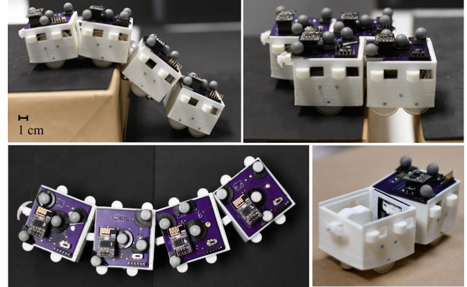
Fig. 1: Top: Robots can form a flexible chain and go down a step (left) or a rigid structure that crosses a gap between two equal-height test stages (right). Bottom left: Four robots forming an articulated chain. Bottom right: One robot inserts its anchor inside the opening of another one (circuitry removed for visual purposes).
