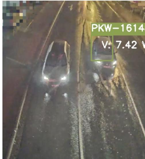
Fig. 1: A snapshot of the camera sensor at the Lemgo intersection on a rainy night, showing that a vehicle was not detected due to poor visibility.
