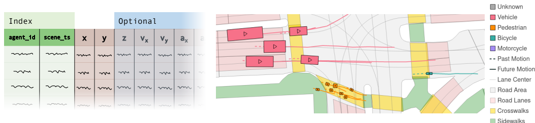
Figure 2: Left: trajdata adopts a tabular representation for trajectory data, leveraging advanced indexing to satisfy user data queries. Right: Agent trajectories from the nuScenes [18] dataset visualized on the scene’s VectorMap, containing all of trajdata’s core map elements.
