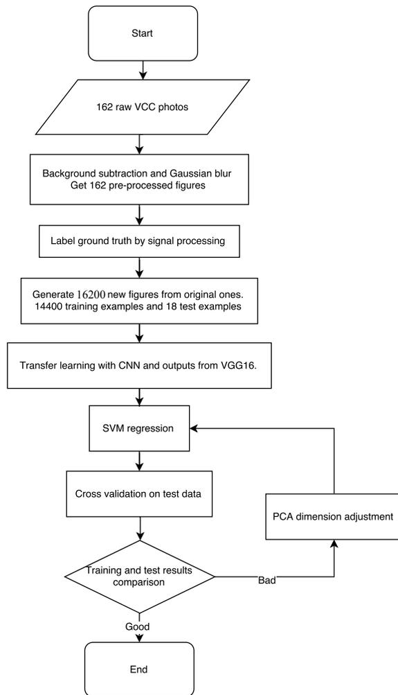
Figure 2: Algorithmic flowchart
