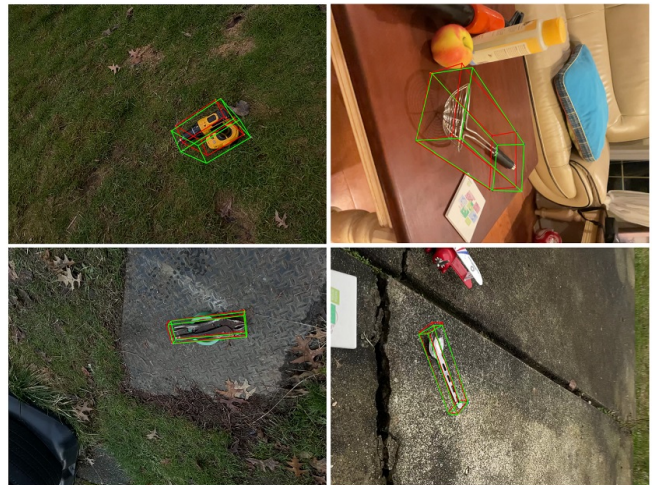
Fig. 6: Category-level object detection and 6-DoF pose estimation results from CenterPose [37] (red) on test images containing unseen object instances, compared with ground-truth (green).
