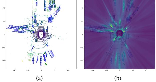
Figure 3: (a) Detection of BEVFormer. (b) The corresponding BEV features of BEVFormer. Since BEVFormer cannot use depth for distinction, the features of each object on the BEV tend to be ray-shaped. The model thus predicts multiple boxes for one object along the longitudinal direction.
