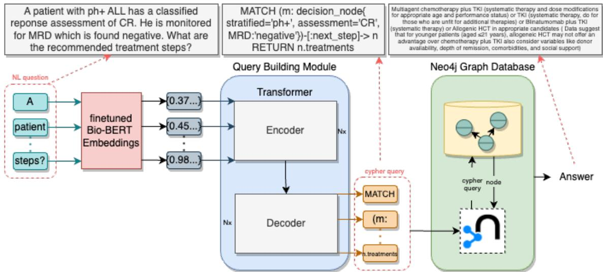
Figure 3: Question Answering using DKG; i) Query Building Module builds the cypher query from given natural language (NL) question, ii) Neo4j Graph Database fetches the node from the DKG according to the query and returns the content of the node
