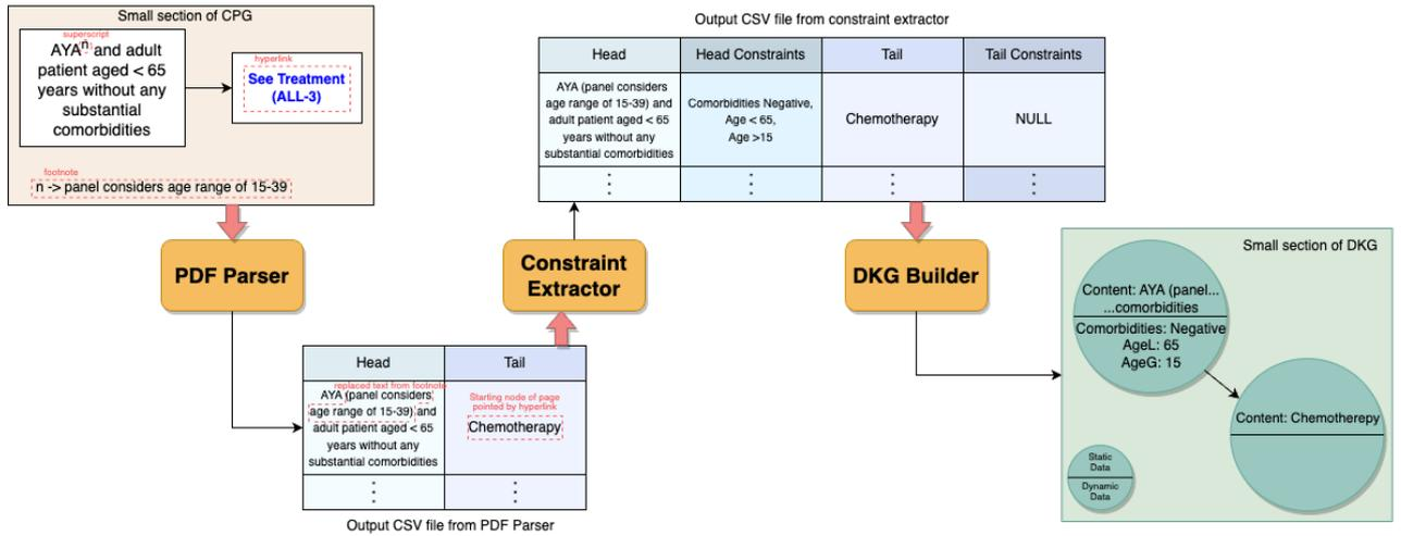
Figure 2: DKG Construction; i) PDF Parser: converts PDF of NCCN guidelines to CSV file, ii) Constraint Extractor: extracts the constraints (refer to Section 3.1 for definition) from each sentence and adds them to CSV file, iii) DKG Builder: takes the CSV and builds the DKG in neo4j graph database
