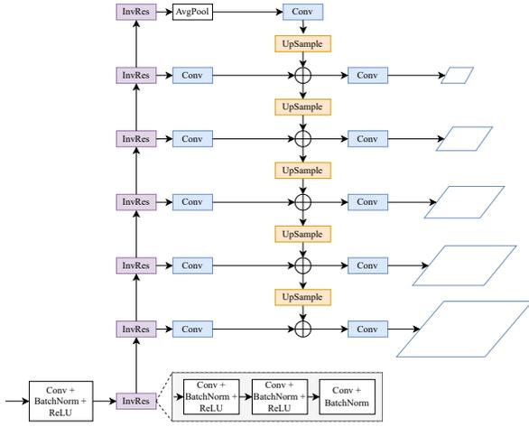
Figure 3: Mobile Feature Pyramid Network architecture
