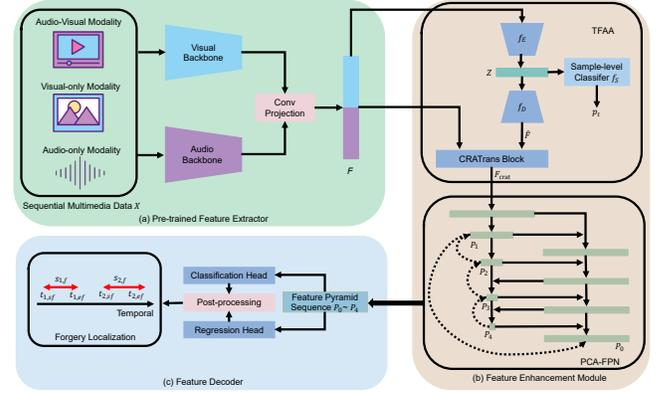
**Figure 2: Illustration of the proposed UMMAFormer, which consists of three main components: (a) a pre-trained feature extractor that maps the sequential multimedia data  $X$  to sequential features  $F$ , (b) a feature enhancement module that enhances the feature representation to multi-scale modified-sensitive features, and (c) a feature decoder that decodes the feature to localize forgeries in the data.**
