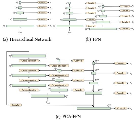
Figure 4: Comparison of feature pyramid networks design in the case of 5 levels.
