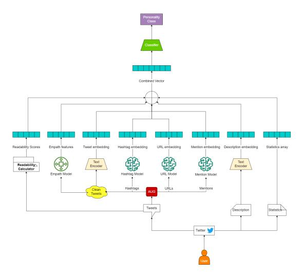
Fig. 5. The overall architecture of our model. The AUG module separates the hashtags, URLs and mentions, and cleans the rest of the tweets.
