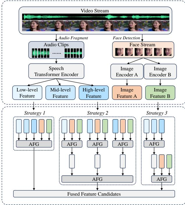
**Figure 1: Deep acoustic and visual features extraction and the following three feature fusion structures. Structure of the attention-guided feature gathering (AFG) module is shown in the following figure.**
