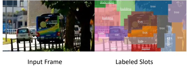
Figure 8. Labeling any slot. The first image shows the input frame. The second image shows the localization of that frame, as well as names for all slots. Slots names with underscore are those having a low cosine similarity.
