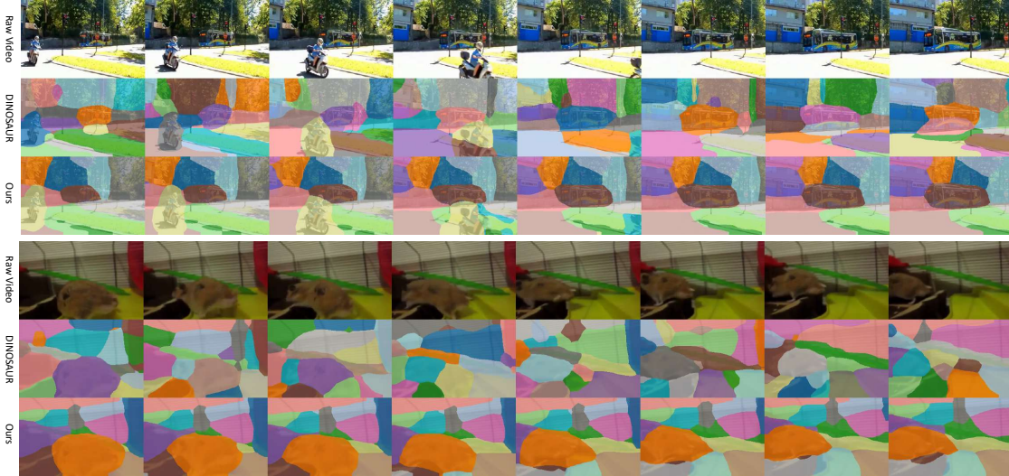
Figure 6. Consistent localization in video. We compare the localization performance from DINOSAUR and ours on two 8-frame video samples. We visualize the spatially interpolated localization for patch-based slot assignment. DINOSAUR is an image-based baseline thus its localization has no temporal consistency. In contrast, ours, as a spatio-temporal localization method, provides temporal consistent localization, as the same region or object are consistently localized by the same slot (indicated by the same color) across frames.
